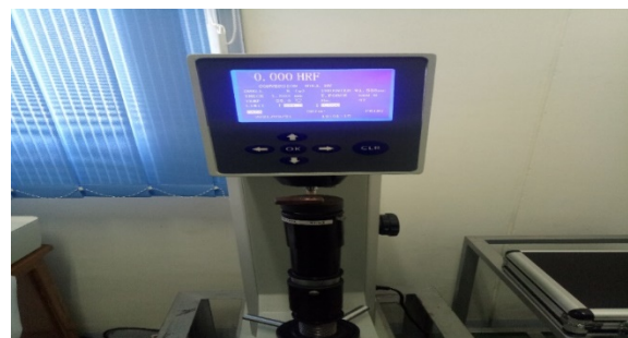
Gambar 5. Alat uji kekerasan, testing machine tipe mtech hardness test
